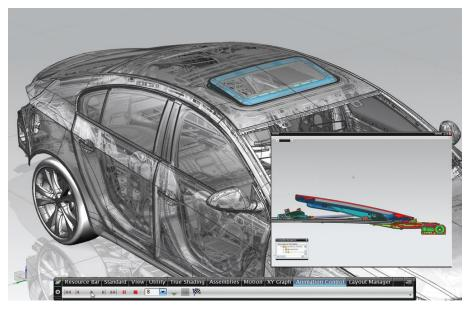
NX Motion handles complex dynamic simulations such as sunroof mechanisms.
