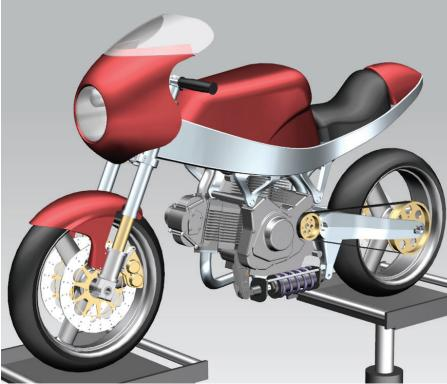
Perform multi-body dynamics on real CAD geometry.
