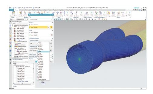
Automatic connection mesh support Simcenter 3D provides a number of solver-supported methods for connecting different meshes together.
